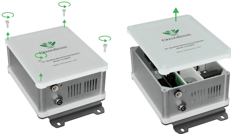
Figure 29: Unscrew the device.
