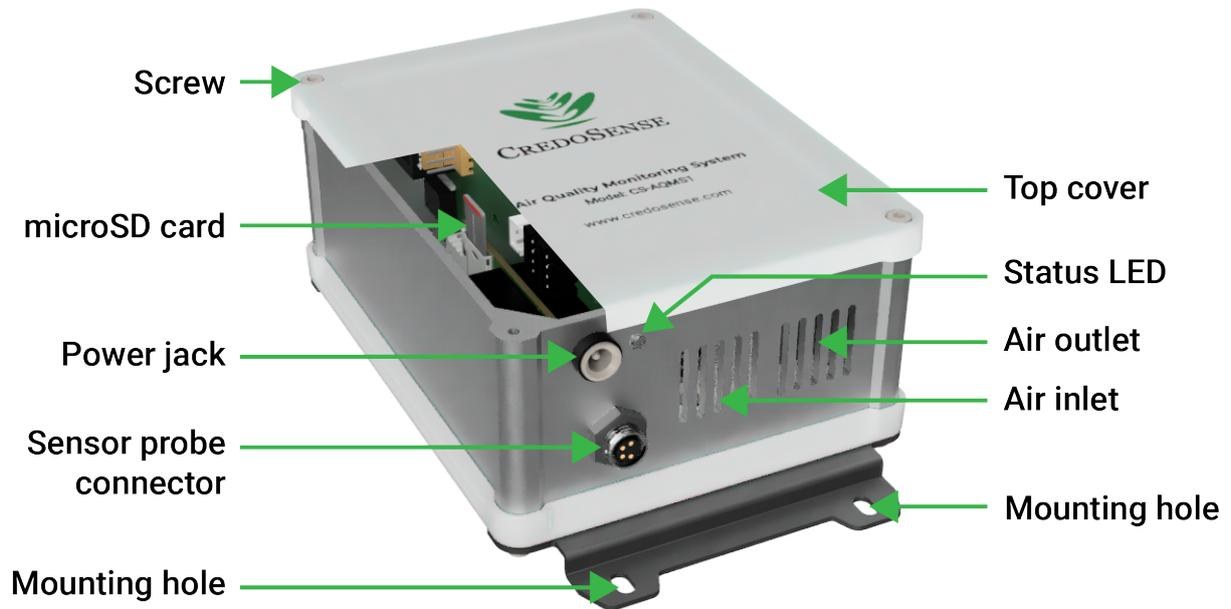
Figure 2: Annotated CS-AQMS1 Structure and Component Overview
