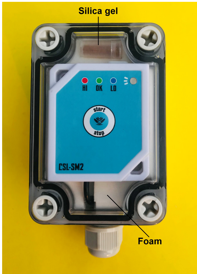
Figure 3.4: Self-logging System is placed in a protective box
