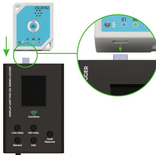
Figure 3: Connecting a CSL-Series Logger.
